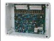
RC-16 is used to operate up to 16 loads at a recycled mode. Option: model RC-16-BT including internal timer (for loads activation depending on mode of external differential-pressure switch).
