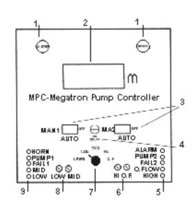
[1] Pushbuttons: H.STOP - buzzer turns OFF; RESET - turns OFF LED's, ALARM and HORN [2] Display 3.5 digits (0-199.9), 1/2" height, LCD
